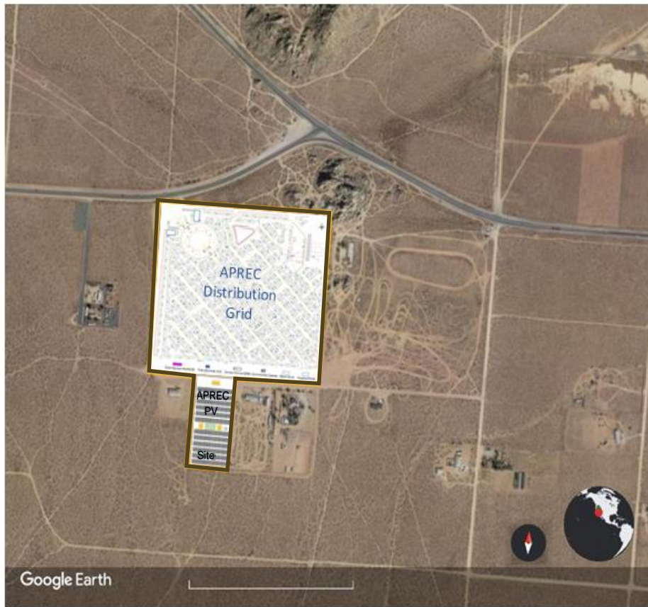
Figure 2.5-1 Preliminary APREC Photovoltaic Generation & Distribution Layout (1:12000 Map Scale, Google Earth 2022)
