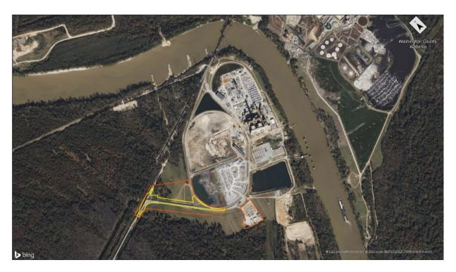
Figure 1-1 Aerial view of the LEC bridge replacement Project area, showing the proposed bridge corridor (in yellow) and potential environmental impact area (in red), including laydown areas.
