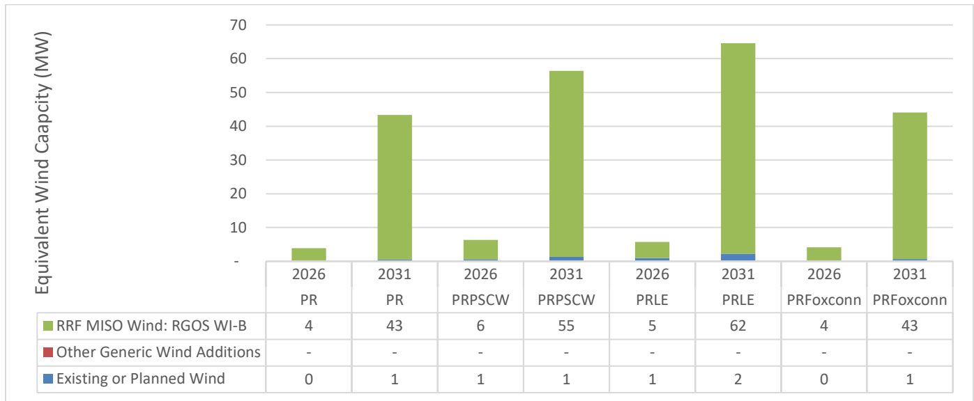
1 Figure S-5-2. Increase in equivalent wind capacity in the Alliant West area due to the Project.
