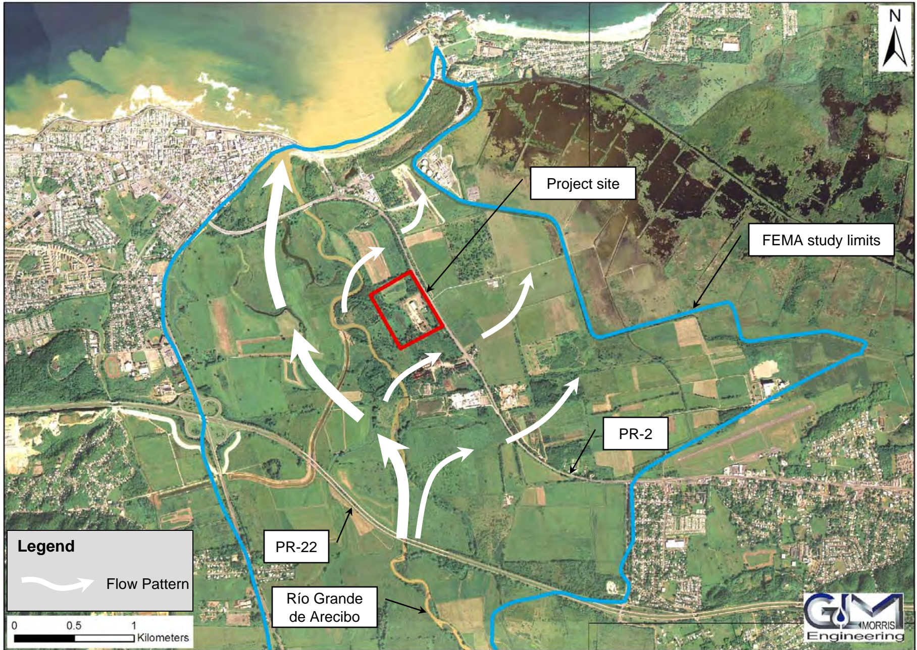
Figure 3: Flow Patterns below Highway PR-22 Bridge.
