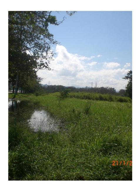
Wet terrain filled by storm water along Road PR-2 outside the Project parcel. The accumulation of water is the result of poor drainage in a canal that serves the said road.
