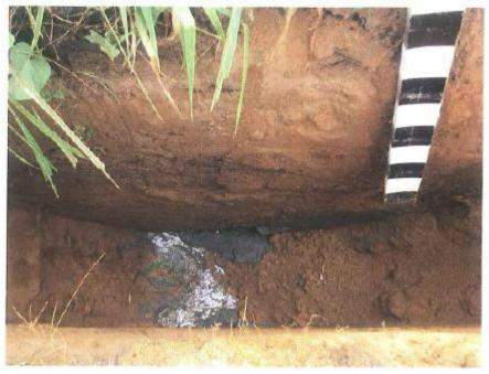
**Photo 15:** Example of trench excavated with heavy machinery, note river sand stratigraphy and water table at the bottom.
