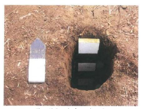
**Photo 12:** Example of manual test pit.
