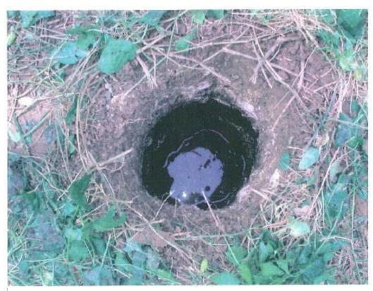
**Photo 8.** Representative test pit, note water table.
