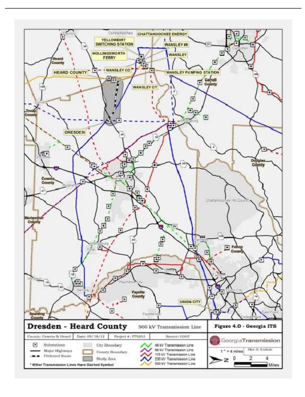
Figure 4 – Georgia Integrated Transmission System Map
