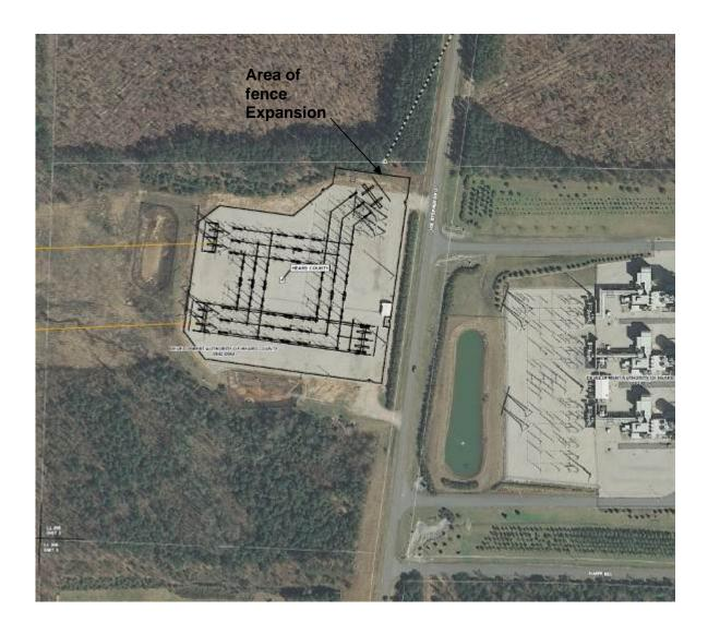
Figure 3 – Heard County Power Substation Modification
