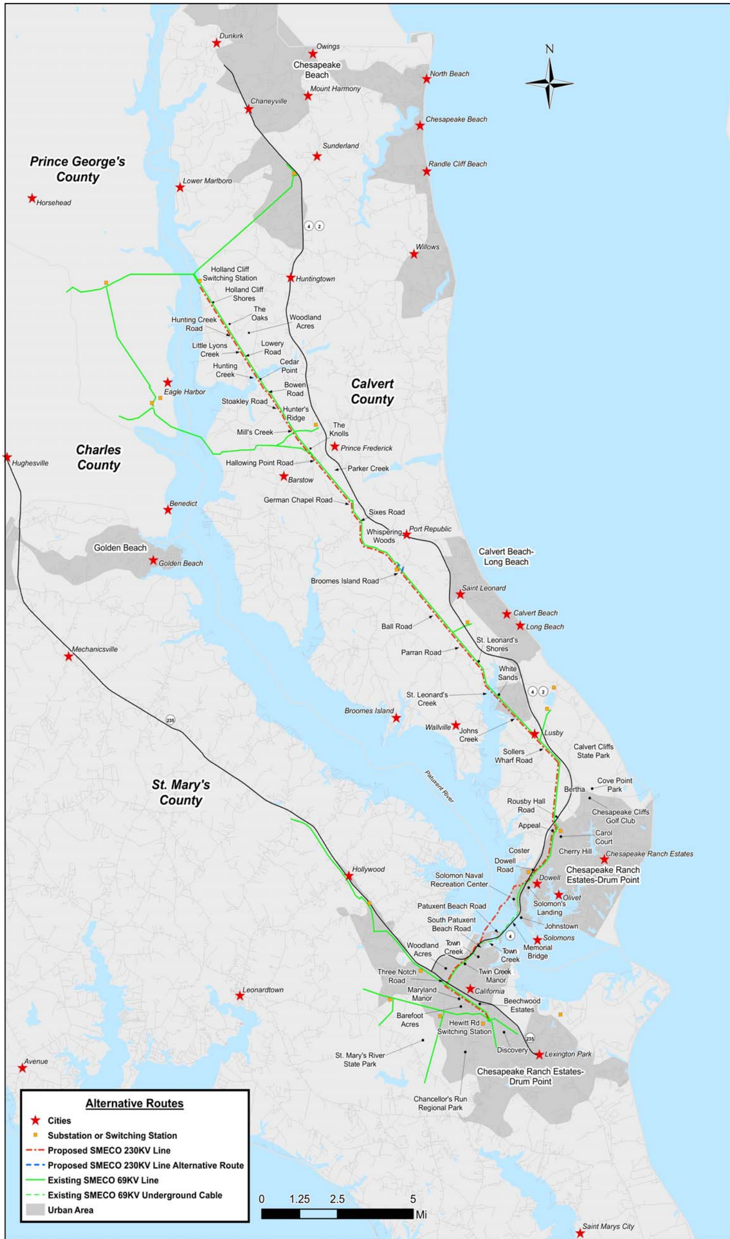
Figure 1-11 Alternative Route Segments for the SMECO Proposed 230 kV Line Source: Black & Veatch
