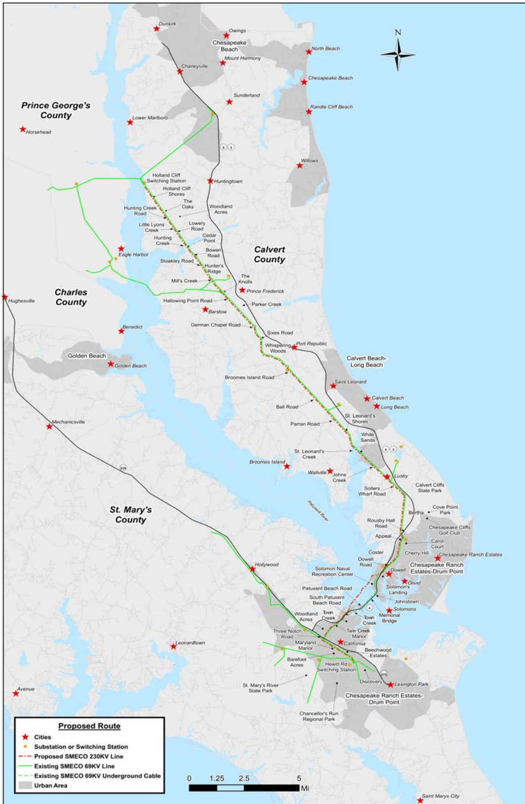
Figure 1-7 Route for SMECO's Proposed 230 kV Line with Cities Neighborhoods and Other Features Source: Black & Veatch
