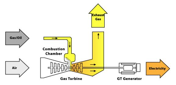
Figure 4-1: Simple Cycle Unit Process Flow Diagram
