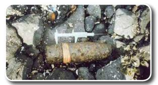
An example of a medium caliber munition
